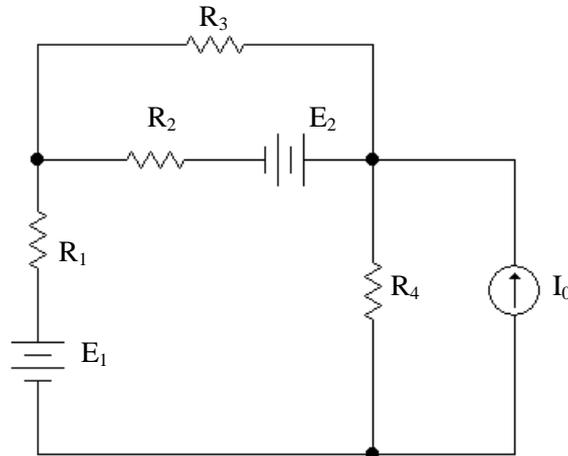
$$\begin{aligned} R_1 &= 22 \text{ k}\Omega \\ R_2 &= 56 \text{ k}\Omega \\ R_3 &= 56 \text{ k}\Omega \\ R_4 &= 33 \text{ k}\Omega \\ E_1 &= 12 \text{ V} \\ E_2 &= 5 \text{ V} \\ I_0 &= 1 \text{ mA} \end{aligned}$$
